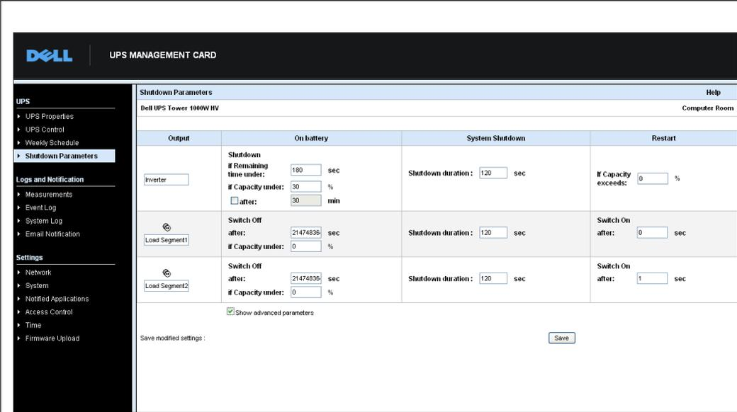
The screenshot displays the 'Shutdown Parameters' configuration page for a Dell UPS. The page is organized into a table with four main columns: Output, On battery, System Shutdown, and Restart. The 'On battery' column is further divided into 'Shutdown' and 'Switch Off' sections. The 'System Shutdown' and 'Restart' columns have their own settings. A 'Save' button is located at the bottom right of the configuration area.
